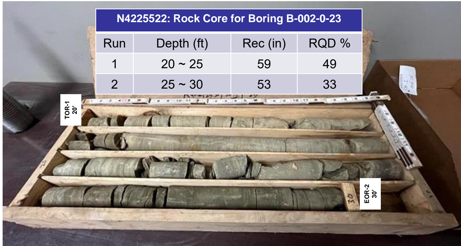
PHOTO 2: ROCK CORE OF BORING B-002-0-23, BOX 1 of 1
